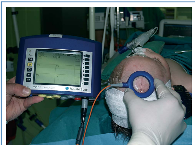
FIGURE 1. Telemetric reading and monitoring device for ICP measurement. ICP, intracranial pressure.
